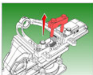
Demontati brida de fixare (brida are 2 suruburi S 17)
