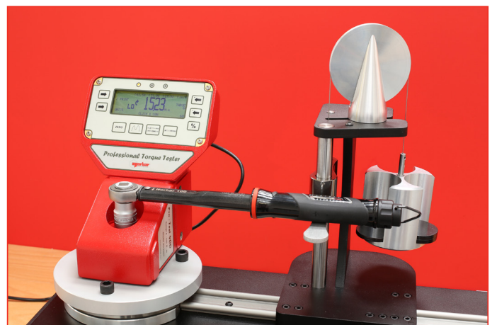
60323 Pro-Test and Static Torque Block Adaptor Kit
