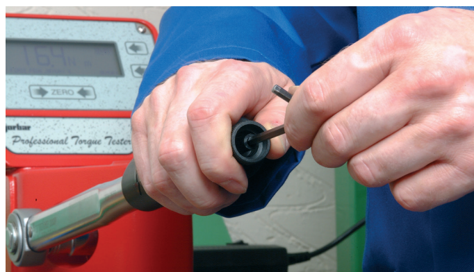
Setting a 'P' Type Torque Wrench
